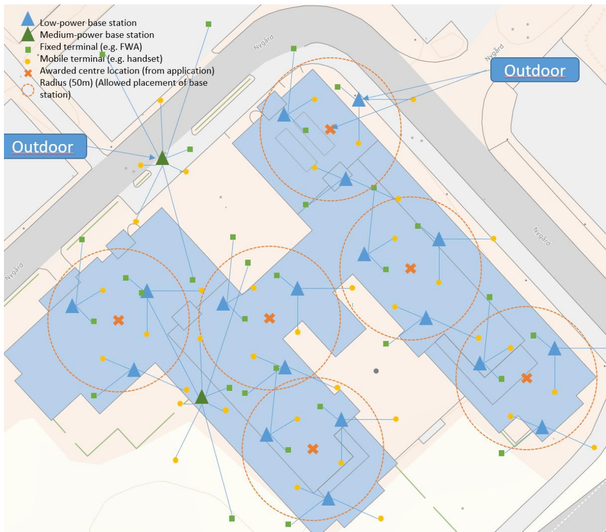
Figure 7: Multiple low-power licence areas combined, and how the uppermost licence area is deemed outdoors (if one or more low-power base stations are outdoors, the entire licence area is deemed outdoors)
