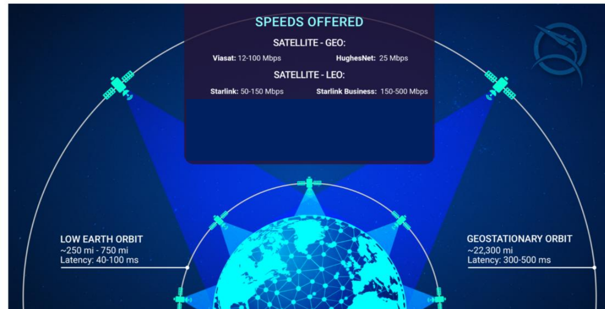
Figure 1.1 Satellite orbit depictions with latency and download speeds – Not to scale
