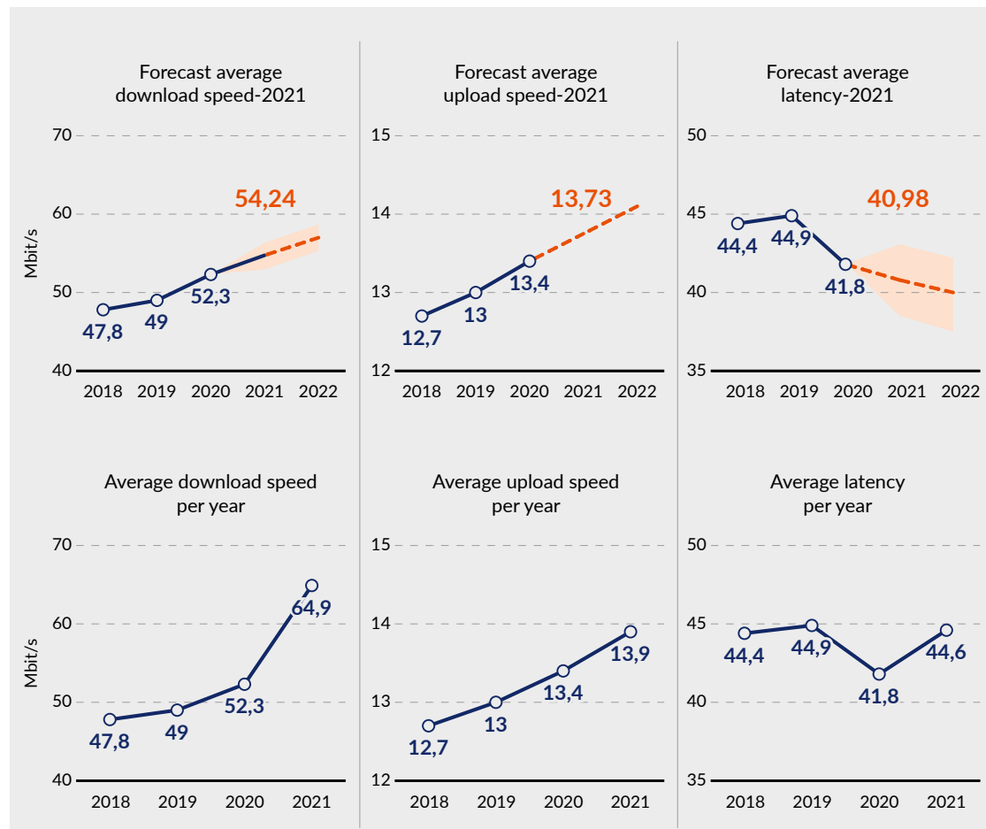
Figure 6: Forecasts of general quality of the internet access service in the 4G mobile networks in 2021. The upper part of the figure shows the forecasts, while the lower part shows the achieved result. (source: Nettfart mobile app)
